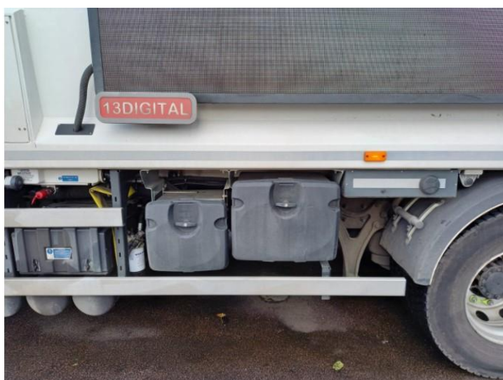
Figure 4-1: Compartment Added to Recycling Collection Vehicle for Small WEEE
