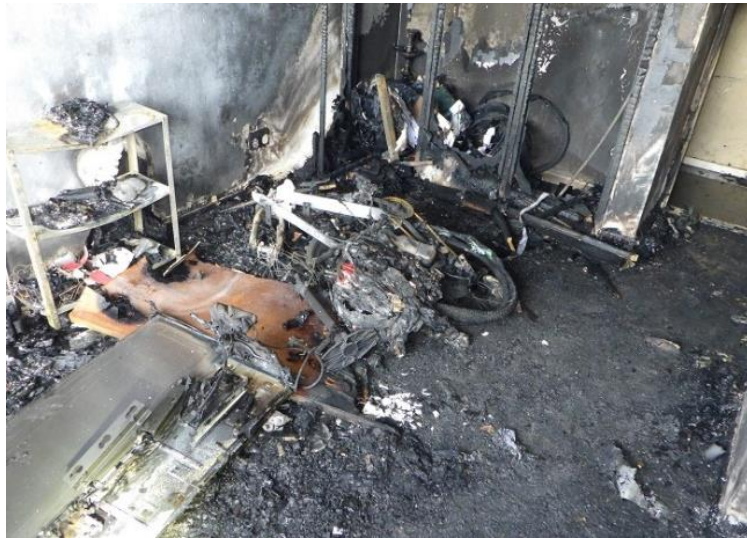
Figure 2: Aftermath of a domestic fire caused by a rechargeable battery (from London Fire Brigade)
