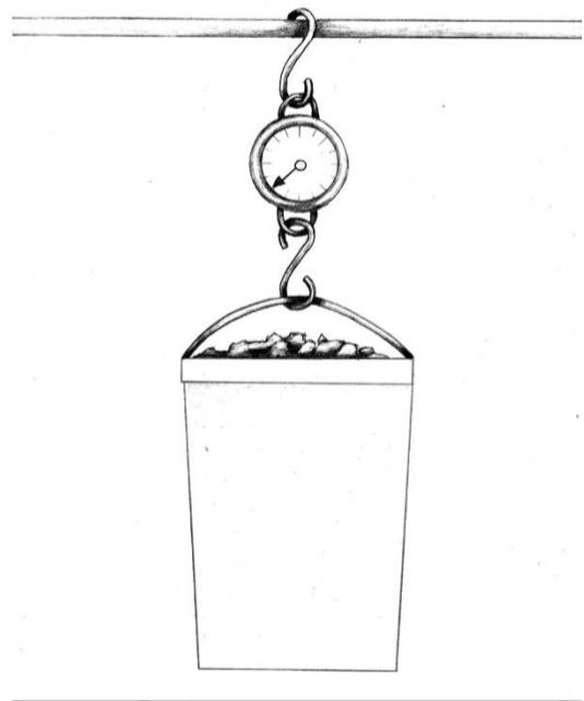
Figure 1-9: Hang the scales from a tree to weigh the full containers.
