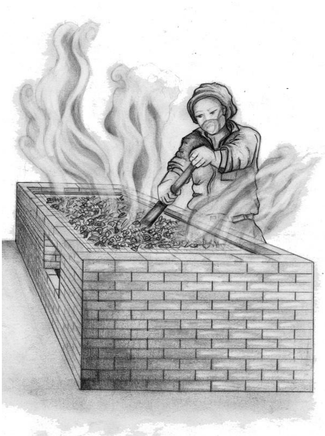
Figure 4-2: Class 2 animal feed is made by smoking and milling fresh fish remains.
